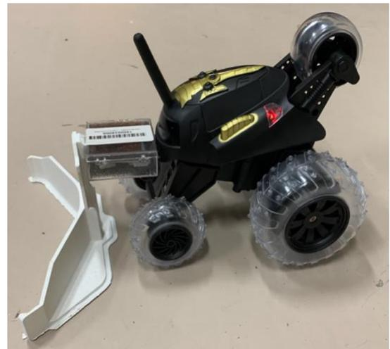
**Figure 2. Boat Prototype** The plow from the NVIDIA robot was 3D-printed and affixed to the front of a remoted controlled car
