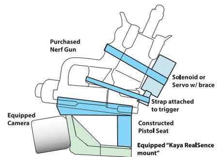
Figure 1. Threat Elimination Tank Modification
